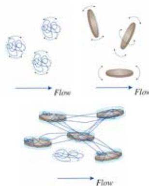
Only C2P08 with shear thickening shows optical anisotropy. The changes in  $\Delta n$  come from clay orientation coupled with PEO.
