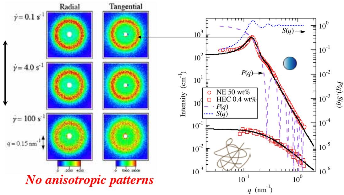
The shape of the NE and the inter-particle distance are preserved and only the long-range inhomogeneities increase by shearing.
