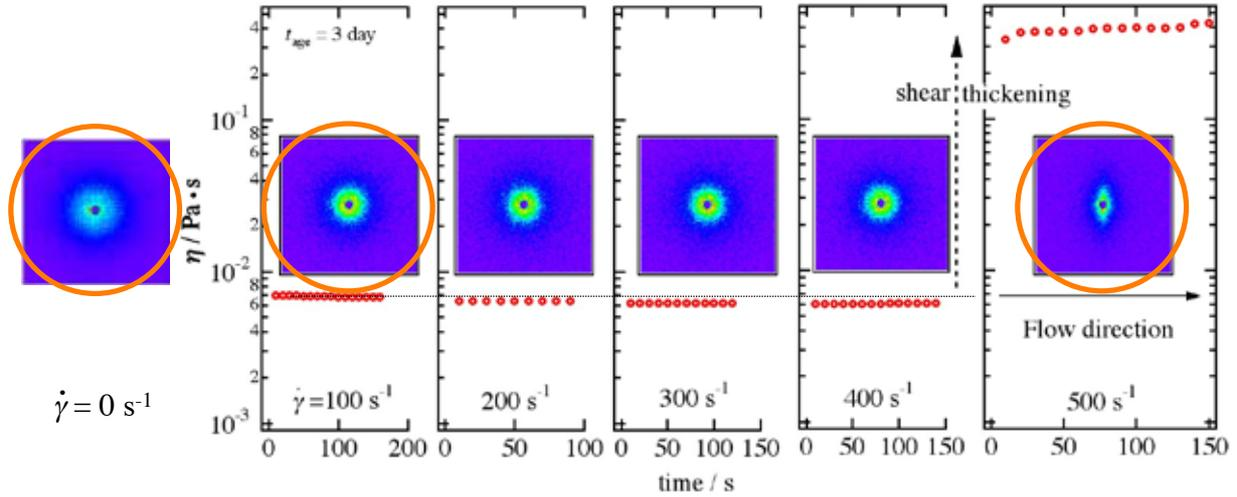
The scattering pattern changed to anisotropic at 500 s<sup>-1</sup>.
