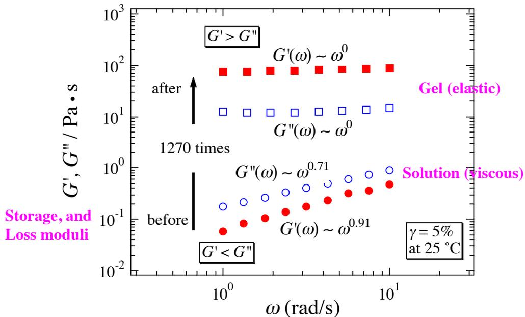
$G'(\omega)$  and  $G''(\omega)$  were measured before and after shearing ( $d\gamma/dt = 100 s^{-1}$  for 10 min)
