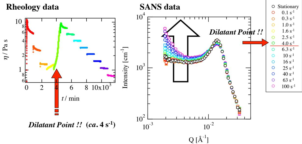
At the shear rate above the dilatant point, a steep increase of the scattering intensity was observed in the low-Q region.
