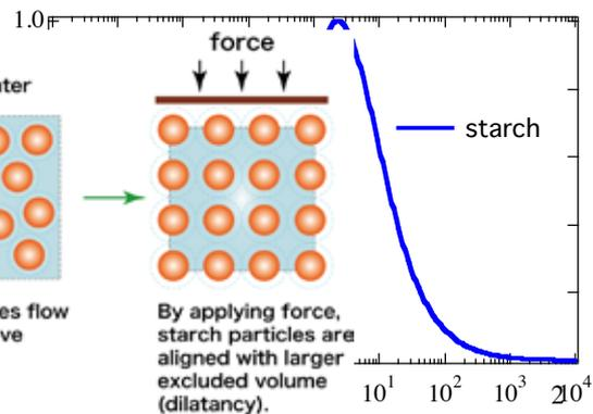
shear thickening of starch suspension
