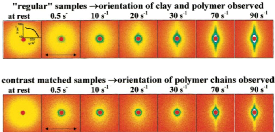
Figure 4. Radial beam configuration: two-dimensional SANS profiles obtained from LRD2 samples in D<sub>2</sub>O (first series, same scaling) and LRD2 contrast matched samples (second series, same scaling).
