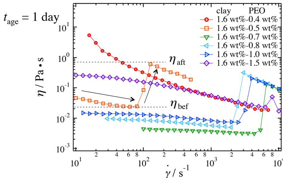
Shear-thickening transition took place at a finite concentration window. The strength of thickening was defined by  $F = \eta_{aft} / \eta_{bef}$
