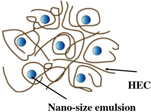
Nano-emulsion was made by high pressure extrusion of 30 wt % glycerol, 3 wt % ethanol, 16 wt % oil.
