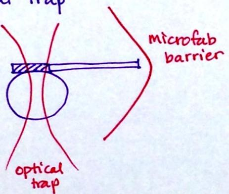
grow into barrier, measure  $\Delta F$ , fix constant  $\epsilon$  by adjusting  $\Delta x$
